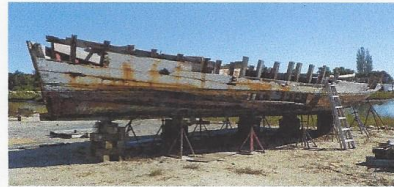
George W Collier at Deal Island Oak frames are holding the boat together. 95% of the boat will have to be replaced
